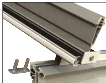
A twin bolt slides into the captivated bolt slot in the eaves beam, prior to the glazing bar being tightened down.
