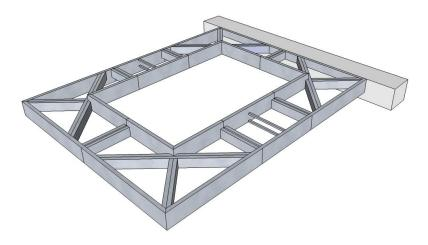
Fix the other rear corner to the ladder rack completing the back section. This will now support itself and the prop can be removed. Take the other sections and continue the assembly until you come to the
