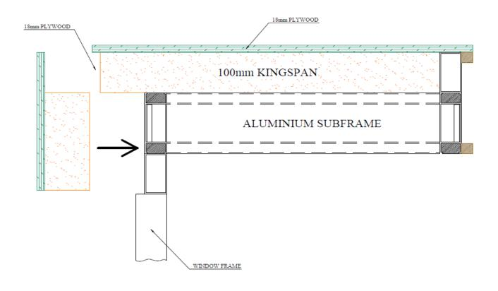
2) The structure can now be decked with 18mm plywood, which is attached using 140mm fixings through the top of the deck, the pre numbered and bonded fascia – ply can then be fixed using 140mm window fixings.
