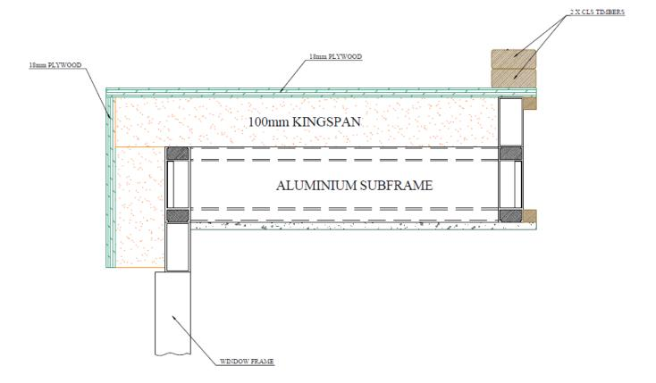
3) An up - stand can now be created using a CLS timber fastened into the box section below.
