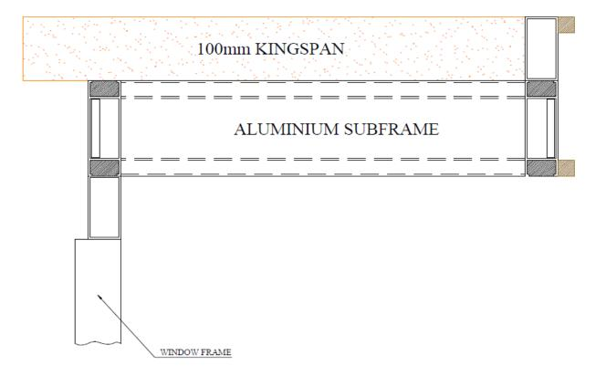
1) Place pre cut insulation on top of the structure as per the numbered plan provided
