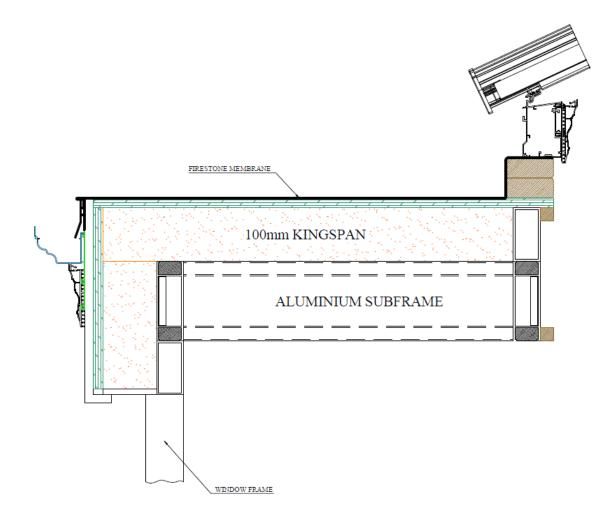
6) Pre assemble lantern roof, apply a generous bead of sealant to the eaves beam perimeter ensuring correct position and fix through into timber kerb at max 450mm centres.
