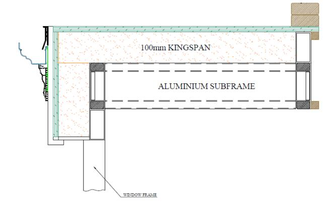
4) Affix soffit & fascia boards (fascia board depth needs to be cut to size dependant on insulation depth). Fix gutter brackets to fascia perimeter at max 500mm centres, trim gutters to length and fit into place. Seat vacuumed formed gutter liners in position using bonding sealant supplied and external cast joiners. Trim heritage cladding to suit and clip on below gutter, bond corner / inline joiners as required,
