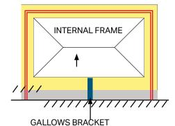
All box beams that support a 265mm fabricated box gutter must be supported by means of gallows brackets, posts or brick piers.
