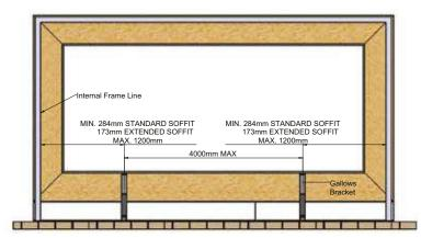
NOTE: Against full height vertical walls, a tapered box gutter would be recommended.
