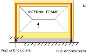
No support is required when using Hup! or brick piers at both ends of the box beam.
