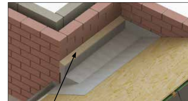
59mm timber packer, lead flash over into tapered box gutter.
