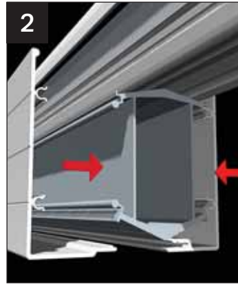
Take the two part cladding, attach each piece carefully to the aluminium bolster profile and 'zip' together.
