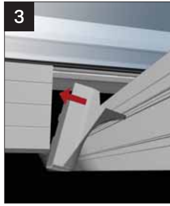
Next take each bolster end cap, simply plug into the PVCu bolster cladding – one at the ridge one at the eaves.
