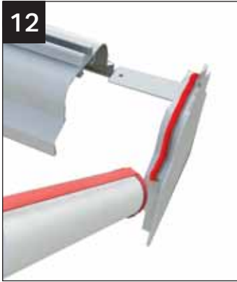
Take the gable end cap, apply sealant as shown and push into ridge capping.
