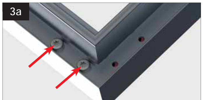
If the pre-drilled holes appear out of alignment as shown above in red simply slacken off the factory fitted screws.
