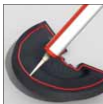
Apply silicone to weather seal as shown. Apply weather seal to glazing, locking wings around ridge - remember, MS Polymer for self cleaning glass (see p38).
