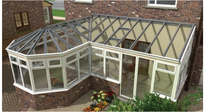
The aluminium rafters, ridges and wall plates are fitted and the spider arms are secured to the spider bracket.
