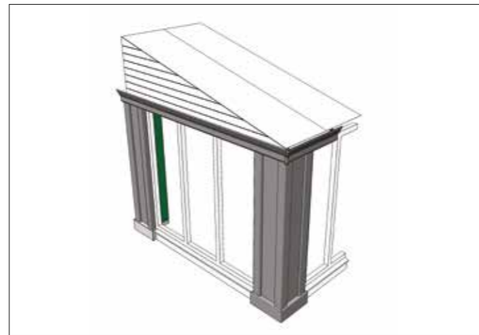
Self manufactured furring with abutment. This design uses Ultraframe's Gable support beam - see illustration B on p31
