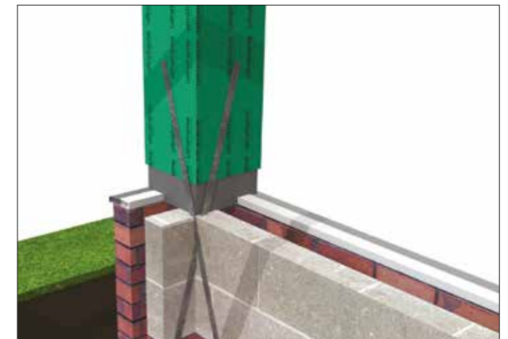
SMALL 90° CORNER Fasten straps down inside of walls of small 90° corner column. Internal brickwork will require grinding to create relief for straps to cross over.
