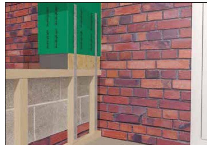
STRAPS MUST LINE UP WITH STUDWORK
