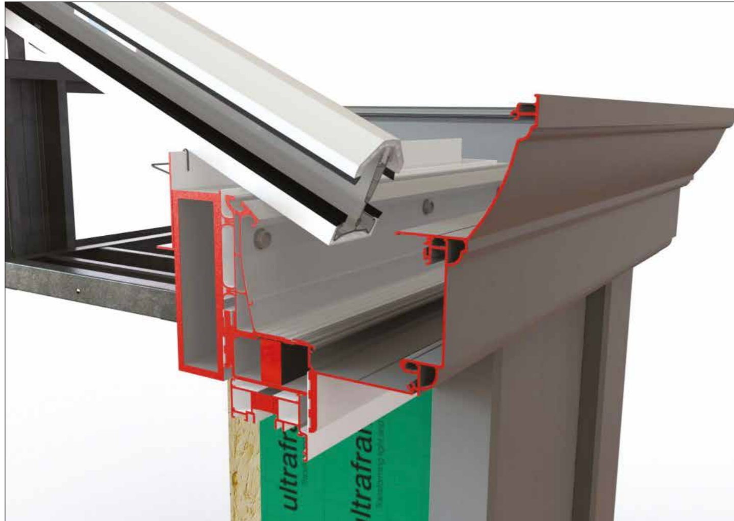
Typical reinforced and bolstered eaves beam ready to accept wide bifolding doors.
